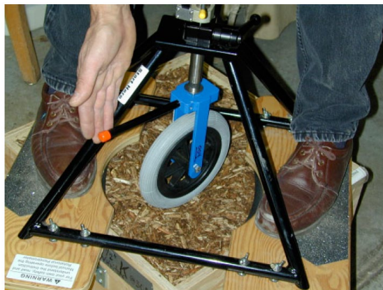
Figure 3—Rotational penetrometer mounted on full-depth playground surface specimen.
